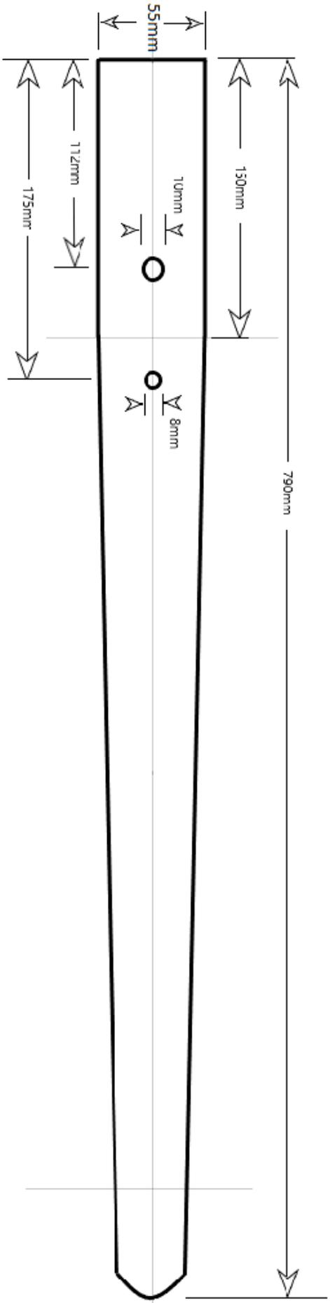
As for the method of attaching the rudder to the boat, I simply took a length of 5mm diameter stainless steel rod, minimum length 180mm, put a thread at either end with a tap and die set, then screwed an eye on one end and a simple retaining bolt at the other. This rod passes through the forward hole on the tiller, the two holes on the bracket and the two holes at the back end of your boat. Poking up on top of the tiller will be the eye, see pictures for clarification.
