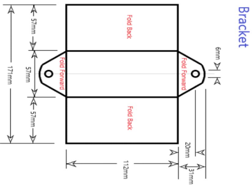
Bracket to be made from 2mm sheet Aluminium.
