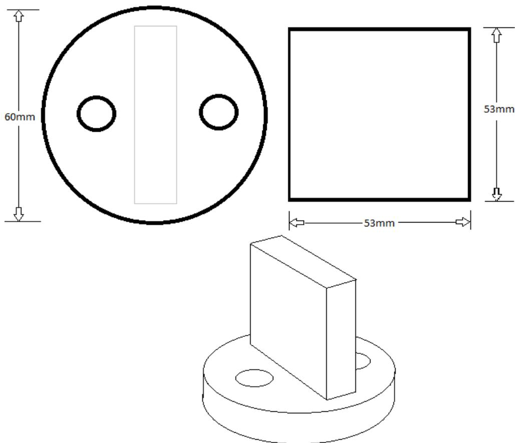
The square part of this stopper slots into the bottom of the mast and you drill a hole in each side of the mast to screw into the upright, remember to bevel the edges of the hole you drill and use countersunk screws so that the screw head does not protrude and eat through the walls of the mast tube.
